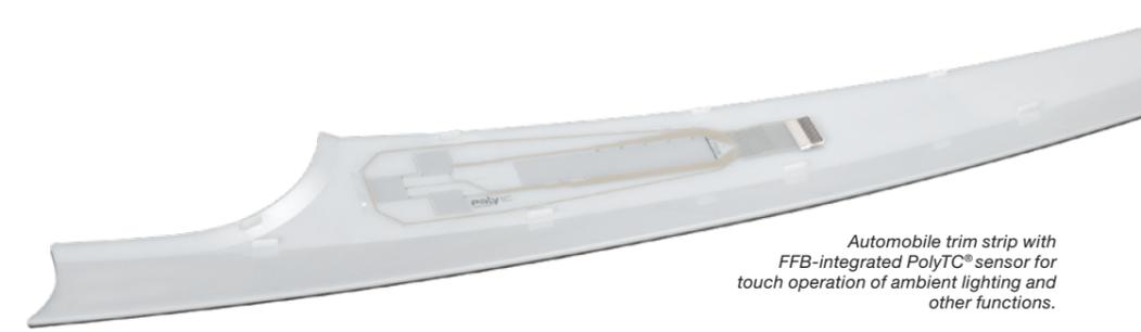
Automobile trim strip with FFB-integrated PolyTC® sensor for touch operation of ambient lighting and other functions.
