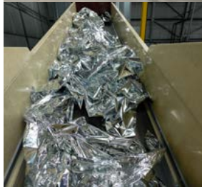
Feeding of residual material into the KURZ recycling plant (RECOSYS® 2.0)
