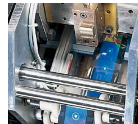
Prägestation / Stamping station
